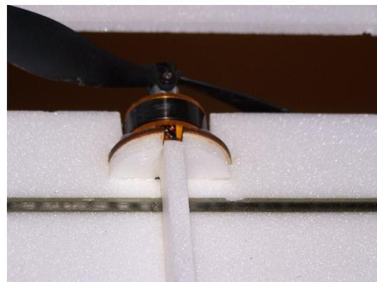
10. Motor Mount. In your kit you should have a ply piece and a little foam disk that match up. Go ahead and laminate them together with some epoxy. Then, mount it to the motor area using epoxy.
