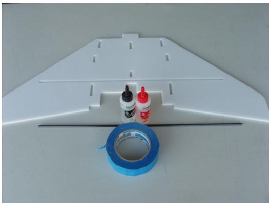
Then flip the wing over, mask on either side of the slot to prevent excess epoxy from getting all over your wing.
