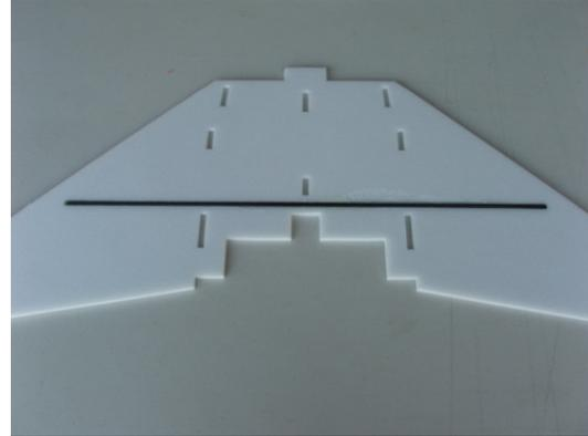
2. Front fuselage assembly. Next, we recommend using epoxy for this step too, it makes the rest of the assembly go a little quicker if you have a nice rigid joint here. Mix up a bit of epoxy and spread on one side of the joint and push it together. Make sure here not to glue to the table again. Really, this happens a lot. **NOTE: Below is what your airplane should look like.**
