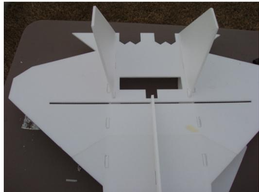
Insert the tail piece into the slots on the top of your model and again, trim a bit to allow some free movement or just work the foam a bit to achieve an outward angle, matching the angle of the intakes. Glue into place. You may want to use epoxy here as well. It is important to get the tails at the same angle, though if they are a little off, it won't matter much. So don't panic.
