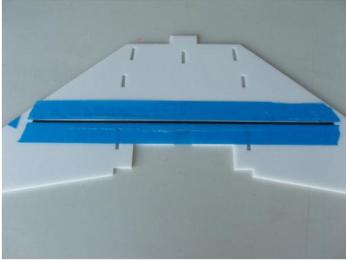
Now, mix up a good amount of epoxy and stir well. The key with epoxy is to really get it mixed well. So mix it like crazy. We recommend using a small cup made of paper or something so you can bend the lip to make like a little spout, but any container will do.
