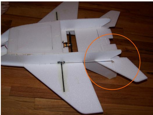
Servo and control horn mounting. This is all about preference. You can mount your servos pretty much wherever, but we prefer under the wing and right over the CF rod. This gets all the wires inside the box on the plane and makes it easy.
