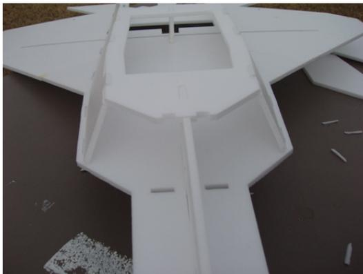
If you flip your plane over, you will notice the tabs extend through the top of the slots slightly. Trim or sand as desired. You can fill in any gaps with
