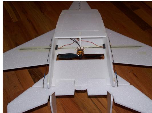
Here (below) you can see the beveled gap in the taileron to allow for free movement positioned on the bottom of the plane.
