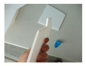
Here (below) you can see the beveled gap in the aileron to allow for free movement positioned on the bottom of the plane.
