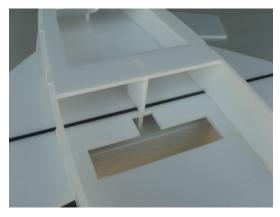
9. Hatch construction. This is the part that might take some creativity on your part. The hatch piece can be attached about a million different ways. Velcro, magnets, and good old fashioned duct tape just to name a few. But you will need to use some scrap pieces of foam to let the hatch stay in place. See below.
