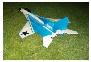
Recommended Set Up. First, what we mean by recommendation. It's what we used and it works well. So you can use a different combo if you like. Also, with just Tailerons, this plane, and all the Quick Builds perform great, but if you really want to increase roll rate, add in some ailerons, just tie them directly to the tailerons and you will be in business.
