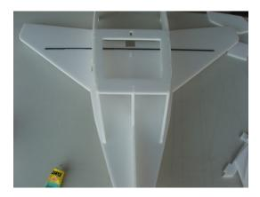
6. Rear Fuselage. Flip your plane over so it's sitting right side up. Find the rear fuselage piece and attach. **NOTE: You can go ahead and mount your motor now, if you complete Step 8 first. It might be easier for you, but not necessary. See step 10 for details.** You will note that there are tabs that fit into the slots.
