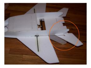
Servo and control horn mounting. This is all about preference. You can mount your servos pretty much wherever, but we prefer under the wing and right over the CF rod. This gets all the wires inside the box on the plane and makes it easy. Study the pictures below.
