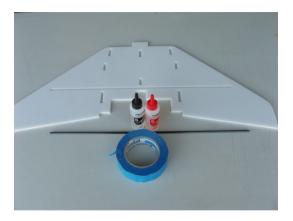
Next, figure out which side of the wing will be the top side. Mask over the slot in your wing using masking tape or painters tape as shown. NOTE: You
