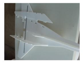
Flip your plane over so the bottom is facing up. You will attach the engine intakes by putting them through the forward most slots as seen in the picture above. You will notice a gentle bend as the intake curves around the body.
